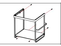
Drill the 4 holes, then insert wall plugs provided. Proceed to secure the frame to the wall using remaining screws provided.
