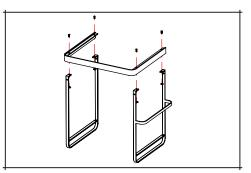
Then using 4 of the matte black fixings provided, assemble the side frames to the top frame.
