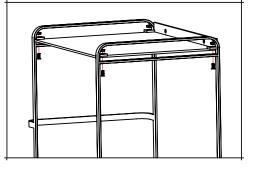
Turn the frame upside down, place on a soft, flat surface. Then using the remaining 4 matte black fixings assemble the shelf to the frame.
