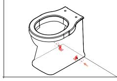
5. With the pan on the desired location, check that the back of the pan fully meets the wall. Remove the pan and further tighten the floor fixings. Return the pan to the desired location paying attention that the pipe fittings are connected with the tubes and secure the screws to the floor fixings through the holes on the sides of the pan. Place the cover caps on the side holes.
