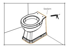
Add sealant around the back of the pan, creating a watertight seal between the pan and the wall.
