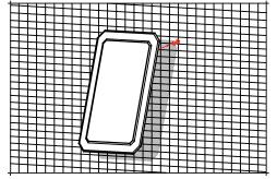
Before hanging the mirror make the electrical connection at the rear of the mirror. Ensure the wires are connected to a switch so the mirror can be turned on/off. Carefully hang the mirror in place, locating the the frame onto the brackets. Ensure the mirror is fully secured onto the mounting holes before letting go.
