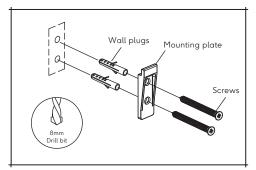
Make sure that there are no hidden pipes or cables in the wall before drilling. Drill 2 holes per mounting plate using a suitable drill bit. The fixings supplied are for solid walls. For hollow or stud walls use specialist fixings. Make sure to align accurately before securing.
