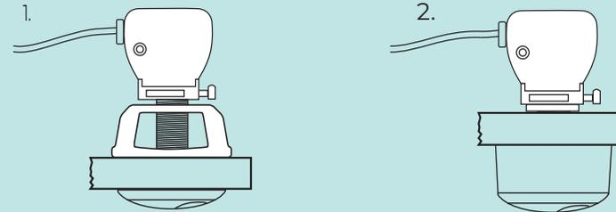
13. If the unit is more than 300mm deep the position of the button can be adjusted to suit. Position the run of the cable as shown below for this application. Note that the hole size is Ø38mm for the button.
