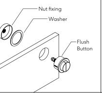
2 -Remove the nut fixing and wash from the flush button and place through the hole. Then orientate the button and add the washer and tighten the nut fixing securly from behind.
