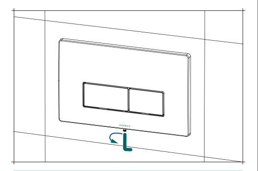
Using the grub screw & allen key provided, tighten the grub screw until it is flush with the bottom of the plate.
