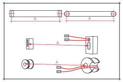
position of the fixing blocks on the wall, ensuring they are level. Drill the holes marked and install the fixing blocks with the plugs and screws provided. The wires should be taken through the fixing blocks.
