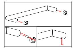
3. Connect the wires to the connection terminal supplied in the towel rail. Gently push the towel rail into the fixing blocks ensuring they go all the way to the wall.
