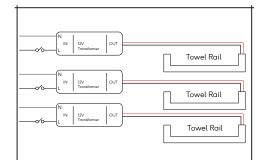
Each towel rail must be installed with the 12V transformer supplied. The distance from the transformer to the towel rail must be **less than 2 metres.**
