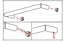
Connect the wires to the connection terminal supplied in the towel rail. Gently push the towel rail into the fixing blocks ensuring they go all the way to the wall.
