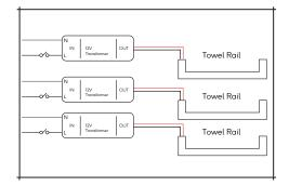
Each towel rail must be installed with the 12V transformer supplied. The distance from the transformer to the towel rail must be less than 2 metres.
