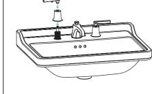
Firstly, you must remove the handle from the valve. Loosen the grub screw on the grip of the handle and slide the grip off the valve. Then remove the small O-ring and unscrew the handle base
