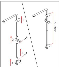
Slide the 'Mount' onto the 'Top riser'. Also slide the 'Shower handset holder' onto the 'Top riser'.
