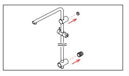
Push the 'Mount' onto the 'Boss' and the 'Diverter' onto the 'Adaptor' and tighten the grub screws.
