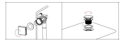
Attach the filler head and waste to the new body.
