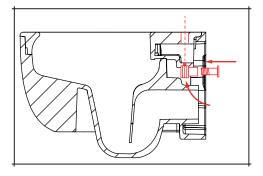
Installing the plastic pan fixings. Firstly locate the round fixing with grub screw on the inside of the pan. align
