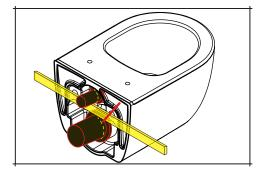
Determine the distance required for the rods on the cistern so that the pan is flush with the back surface. (Measure distance 'X' and translate to 'Y'). Place the new toilet on the wall through the carrier holes. Apply soapy water to the inlet and outlet pipes to help with the connection to the cistern.
