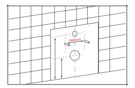
Make sure the water supply is switched off before installing the new toilet. Install the concealed cistern system in the wall, according to the cistern's installation instructions.
