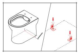
4. With the pan in location, mark the position of the holes on the floor. Measure the ceramic thickness of the pan and mark the approximate location of the floor fixings. Drill a hole on the ground and locate the plugs so they are flush with the ground. Tighten the floor fixings.
