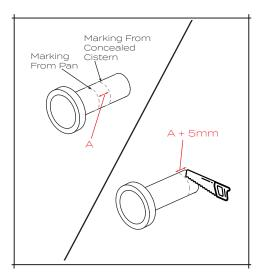
2. Place the Inlet and outlet pipes on the Wc pan and mark where they extend past the edges of the bowl. Then place the pipes completely onto the cistern and mark them where they emerge from the unit. Measure the space between the marks on the pipes (distance A), carry this measurement over to the end of the pipes, adding 5mm and then cut off the end. Use a file to smooth the pipe ends, before securing the pipes into the cistern unit.
