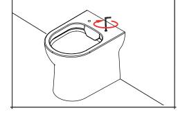
7. Install the seat according to the fitting instructions included in the seat's box.
