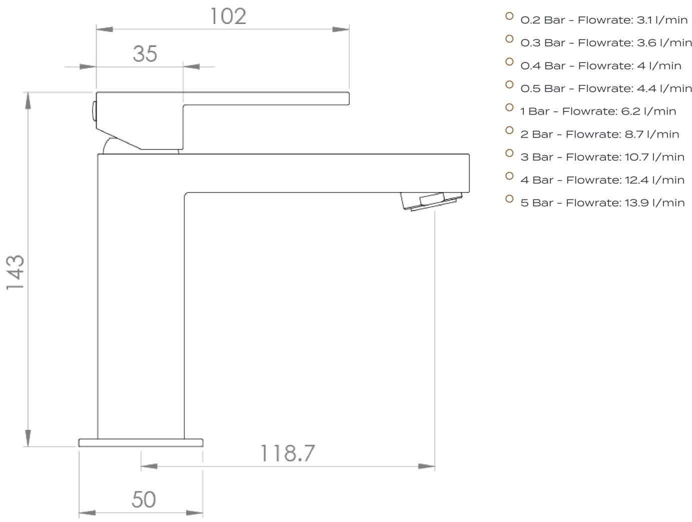
O.3 Bar - Flowrate: 3.6 I/min O.4 Bar - Flowrate: 4 I/min O.5 Bar - Flowrate: 4.4 I/min O 1 Bar - Flowrate: 6.2 I/min
