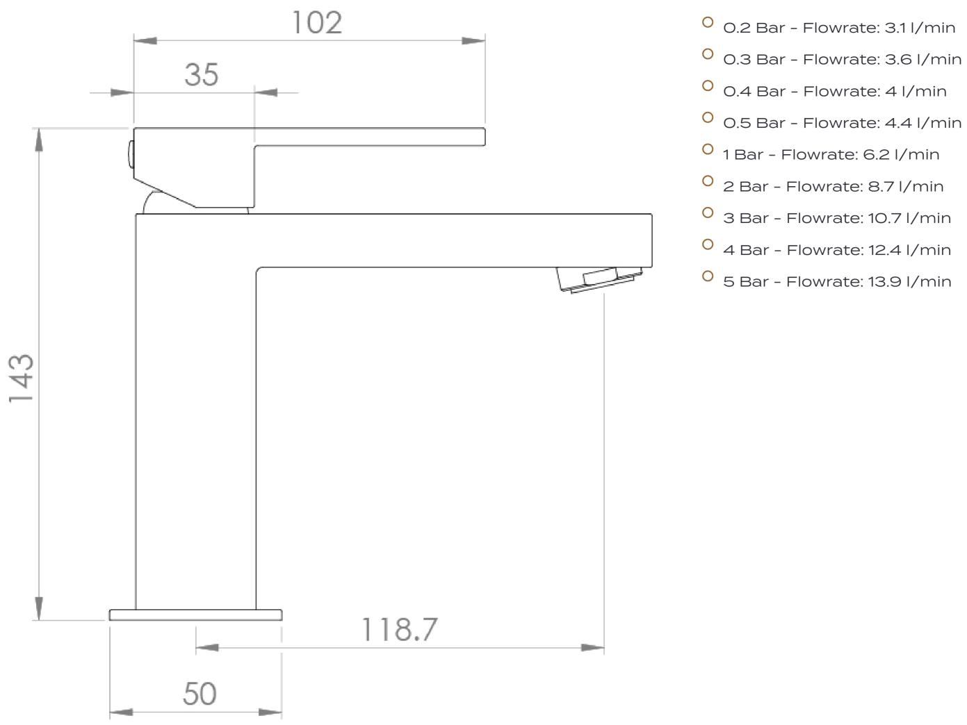
O.4 Bar - Flowrate: 4 I/min O.5 Bar - Flowrate: 4.4 I/min O 1 Bar - Flowrate: 6.2 I/min O 2 Bar - Flowrate: 8.7 I/min O 3 Bar - Flowrate: 10.7 I/min O 4 Bar - Flowrate: 12.4 I/min
