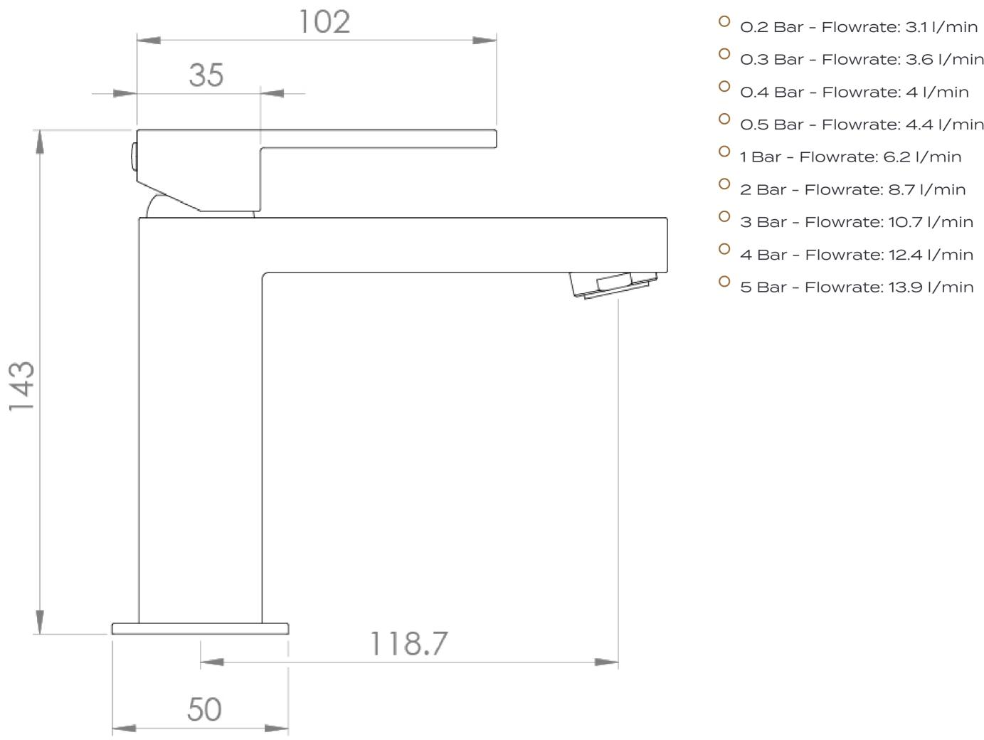
O.3 Bar - Flowrate: 3.6 I/min O.4 Bar - Flowrate: 4 I/min O.5 Bar - Flowrate: 4.4 I/min O 1 Bar - Flowrate: 6.2 I/min O 2 Bar - Flowrate: 8.7 I/min
