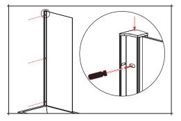
Once the screen is perfectly level in all directions, drive the 3.5mm crews and screw clips provided through both profiles, **avoiding the glass.** Cover the screw head using the screw caps.
