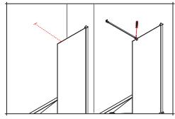
Measure the distance between the wall and glass. Mount the support arm, ensuring a tight fit.
