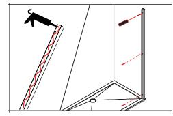
Apply a generous bead of silicone sealant to the back of the profile.
