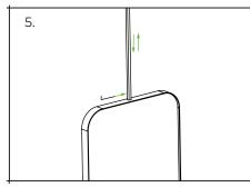
5. Once the mirror is secured to the wall, adjust the upper tube to meet the ceiling and tighten the grub screw.
