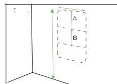
1 & 2 Before positioning the mirror, mark and fix the supports to the wall. Ensuring they are horizontal using a spirit level.
