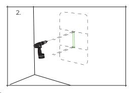
3. For each mounting plate drill two holes in the marked positions using a 8mm drill bit to a depth of 55mm.
