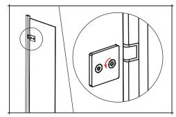
The flipper panel can be adjusted by the hinges. Rotate the wheels behind the hinges to adjust the distance between the flipper panel and the main panel.
