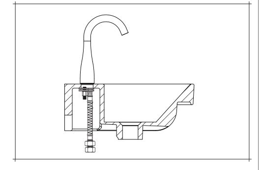
Single lever mixers are fixed using either one or two threaded rods, and a pair of washers. Make sure the rubber washer is closest to the basin and tighten the nut/s until the tap is secure.
