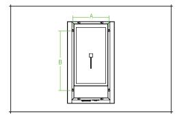
Choose the orientation for the mirror, then measure distance A & B. Mark the 4 points on the wall, ensuring that the holes are level.
