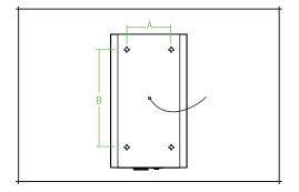
Choose the orientation for the mirror, then measure either distance A & B. Mark the 2 points on the wall, ensuring that the holes are level using a spirit level
