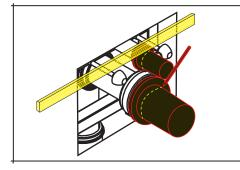
Then place the inlet and outlet pipes completely onto the cistern unit and mark them where they emerge from the unit.
