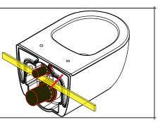
Place the inlet and outlet pipes on the bowl and mark the pipes where they extend past the edges of the bowl.
