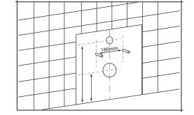
Make sure the water supply is switched off before installing the new toilet. Install the concealed cistern system in the wall, according to the cistern's installation instructions. Measure the pan and set the spacing of carrier studs, tightening the nuts.
