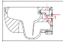
Determine the distance of the rods on the cistern so that the pan is flush with the back surface.
