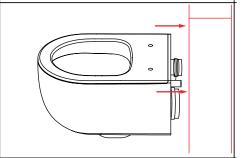
Then place the inlet and outlet pipes completely onto the cistern unit and mark them where they emerge from the unit.
