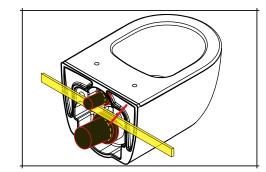
Place the new toilet on the wall through the carrier holes. Apply soapy water to the inlet and outlet pipes to help with the connection to the cistern.
