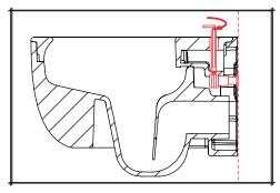
Use the provided allen key to tighten the fixings, making sure the toilet is level. Secure the grub screws as tightly as possible.
