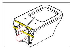
Place the Inlet and outlet pipes on the Wc pan and mark where they extend past the edges of the bowl.
