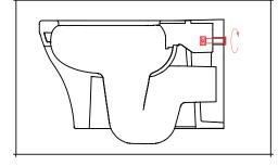
Install the fixing kit onto the back of the pan.
