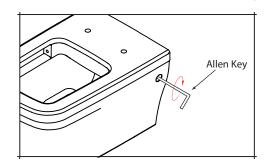
Place the pan on the wall through the carrier holes and bolts on the framed cistern.
