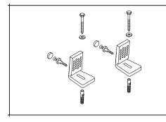
With the pan in the desired location, mark the position of the holes on the floor. Measure the ceramic thickness of the pan and mark the approximate location of the floor fixings. Drill a hole on the ground and locate the plugs so that they are flush with the ground surface. Tighten the floor fixings.
