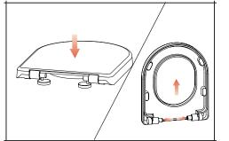
Tighten the screws fully and place the stainless steel cover plates on the hinge anchors. From the upright position, allow the seat to close on its own and check that the soft closing action is working correctly.
