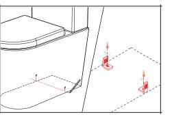
With the pan on the desired location, check that the back of the pan fully meets the wall. Remove the pan and further tighten the floor fixings. Return the pan to the desired location and secure the screws to the floor fixings through the holes on the sides of the pan.
